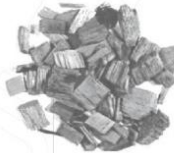
b) Hog fuel (crushed with blunt tools)
